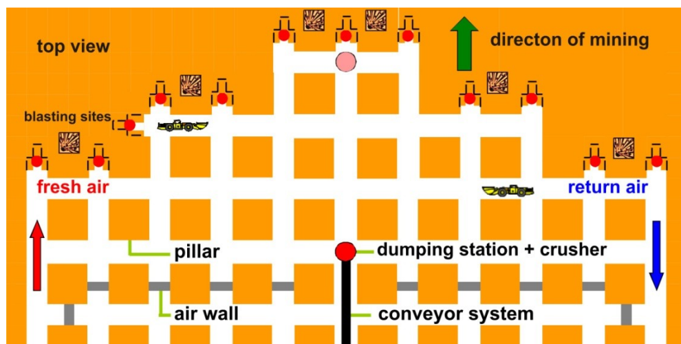
Figure 10: Floor level with 12 blasting sites (source K+S)
